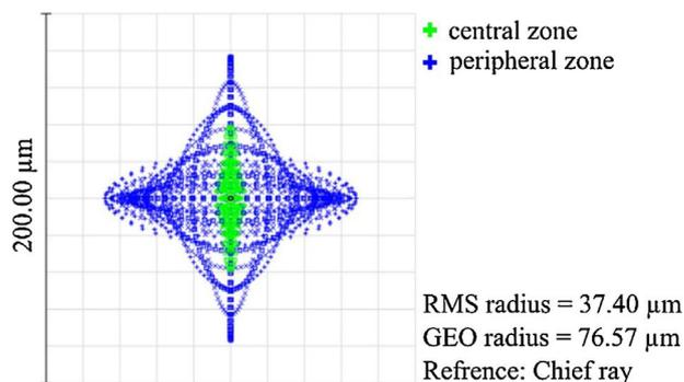
Fig. 2. Spot diagram in the image plane (retina) of the astigmatic eye model corrected with a center near bifocal contact lens. Green and blue symbols represent rays from the central and the peripheral zone, respectively. (For interpretation of the references to colour in this figure legend, the reader is referred to the web version of this article.)
