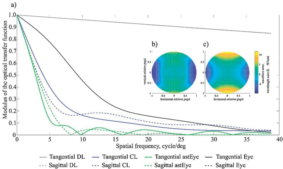
Fig. 3. (a) Image quality analysis of the MTF for the tangential and sagittal image plane of the diffraction limited (DL), the naked model eye (Eye), the astigmatic model eye (astEye) and the corrected model eye (CL). (b) and (c) represent the wavefront error maps (in wave units  $\lambda = 546 \text{ nm}$ ) of the corrected and the astigmatic model eye, respectively.
